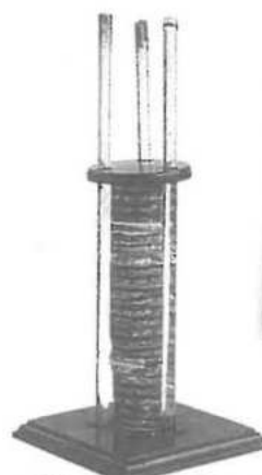
1 The first electric battery
